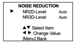
NR2D Level (2D Noise Reduction): Auto, Off,  $1 \sim 5$ . NR3D Level: (3D Noise Reduction): Auto, Off,  $1 \sim 8$ .
